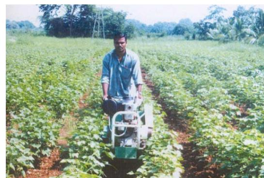
The rotary weeder consists of three rows of discs mounted with 6 numbers of curved blades in opposite directions alternatively in each disc. These blades when rotating enable cutting and mulching the soil. The width of coverage of the rotary tiller is 500 mm and the depth of operation can be adjusted to weed and mulch the soil in the cropped field.
