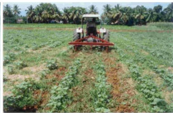
An inter cultivator cum earthing up equipment was developed and fitted to a standard tractor drawn ridger. Three number of sweep type blades are affixed to the ridger frame for accomplishing the weeding operation in between standing rows of crops. Three ridger bottom fitted behind the sweep blade, work on the loosened soil mass and aid in earthing up by forming ridges and furrows. Weeding efficiency is 61 per cent.
